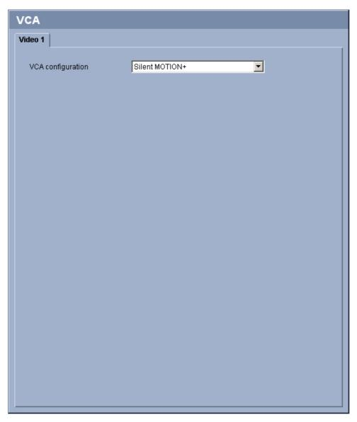
The VOT-320 contains an integrated video content analysis (VCA), which can detect and analyze changes in the signal using image processing algorithms. Such changes can be due to movements in the camera's field of view.
